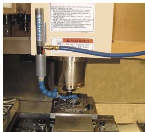
The Model 5315 Cold Gun cools a two foot 3/8" carbide cutter on a CNC, increasing tool life by 50%.
