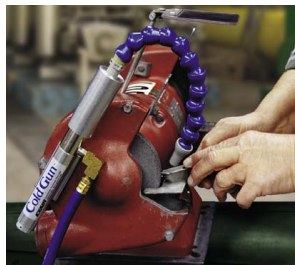
Cold air eliminates heat cracking of the carbide tool during sharpening.
