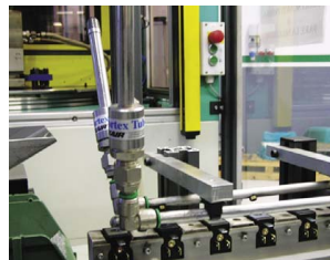
A pair of medium vortex tubes cool a solenoid coil after a welding operation.
