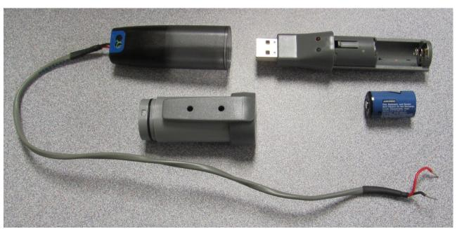
Part 1 – Removing the data logger from the data logging harness and inserting the battery.
